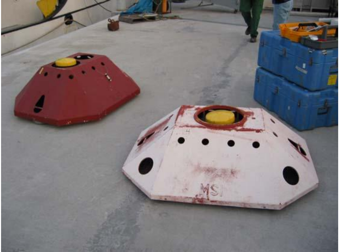
Figure 6. A trawl-resistant bottom mount containing an acoustic Doppler current profiler. Photograph by the Woods Hole Group.
